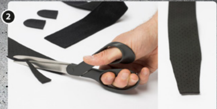
2 Cut down the sides of one end of the strap so its 25–30 mm wide.
